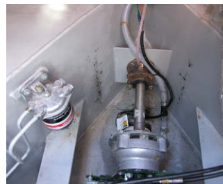
The bilge pump sits in a sump under a conventional stern tube gland. A fuel filter helps reduce potential contamination issues.
