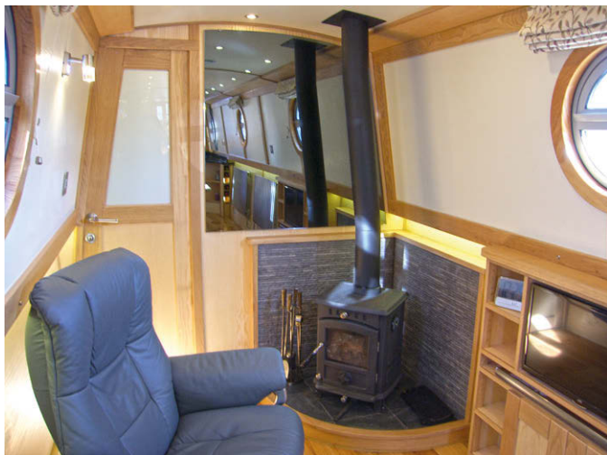
The good-sized solid fuel stove is set on a hearth that complies with the code of practice.
