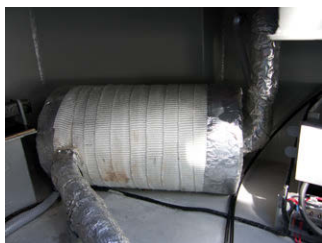
A large attenuation silencer combined with excellent sound insulation under the deckboards makes for a very quiet boat.
