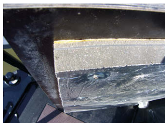
A large attenuation silencer combined with excellent sound insulation under the deckboards makes for a very quiet boat.
