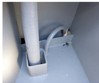
Nice Colecraft detailing: the locker drain is separate from the cockpit drain, and a vent from the water tank is directed overboard.
