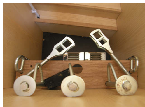
Superb windlass and mooring gear storage in the aft hanging locker – and ventilation into the cabin bilge.
